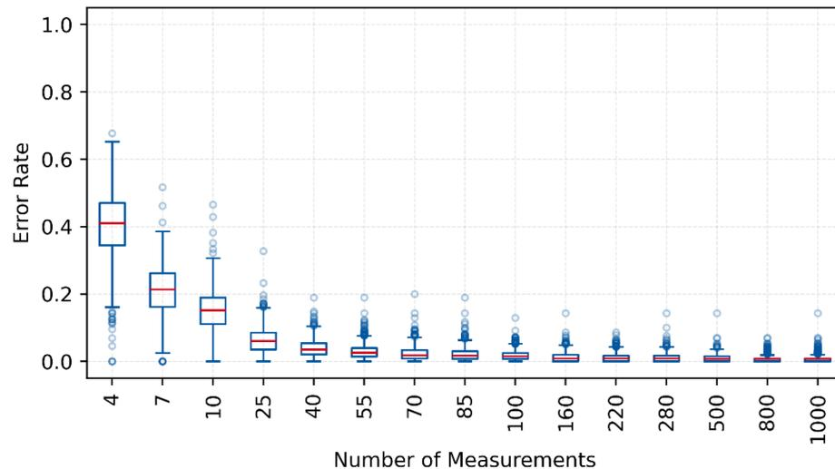
Error rate of topology detection as a function of the number of measurement data
