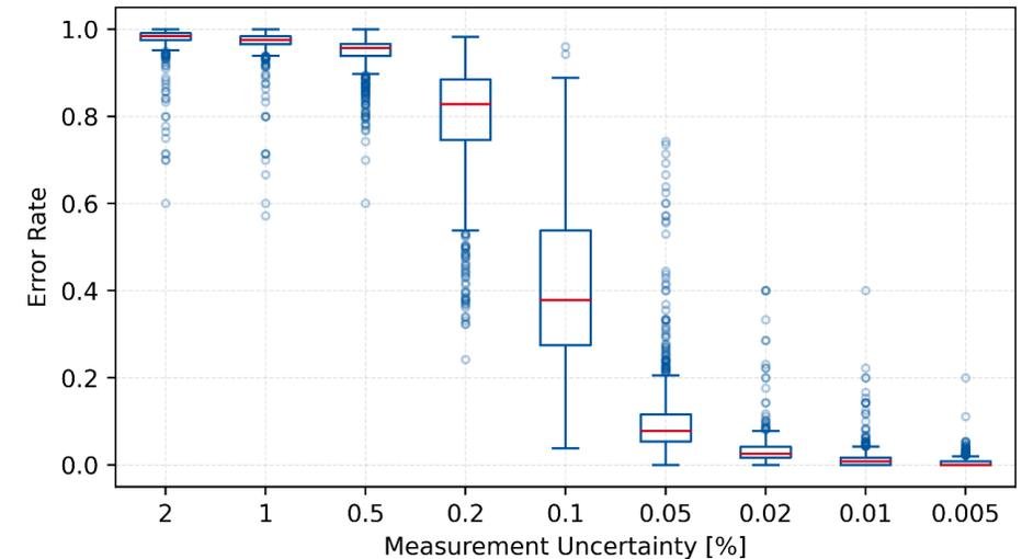
Error rate of topology detection as a function of the statistical measurement uncertainty
